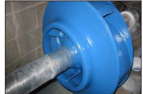
Impeller protected with ARC 855
